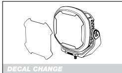
Peel off the adhesive backing of the decal and align the decal to the edge of the lens cover decal outline. Press the decal down firmly and push out any bubbles, Wipe lens cover to avoid decal peeling off when washing
