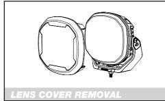
1 Remove Lens Protector by un-clipping the side wings
