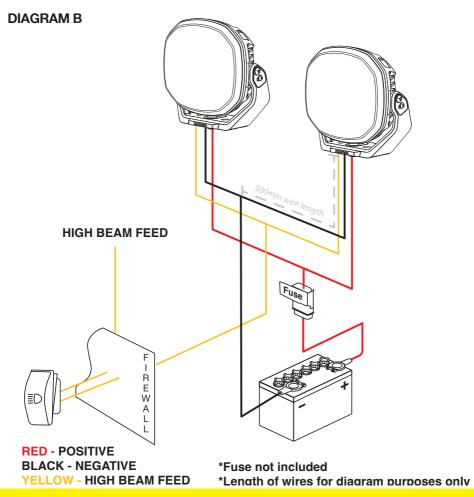
Please consult a qualified Auto Electrician to adapt to your vehicle wiring as wrong connections can cause damage to your vehicle wiring and electronic modules.
