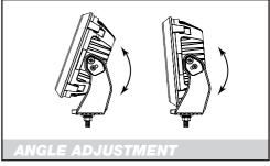
Loosen the nut and adjust lamp to the desired angle. Re-tighten nut
