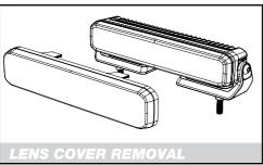
1 Remove Lens Protector by un-clipping the side wings
