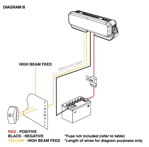
No relay required due to internal switching technology (patent pending)
