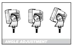
Loosen the nut and adjust lamp to the desired angle. Re-tighten nut
