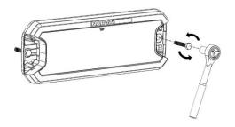
\*\*WARNING: Load resistor must be mounted to metal a surface. Operating temperatures can reach up to 170° C, and will damage plastics, carpets and painted metal surfaces\*\*
