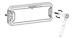
\*\*WARNING: Load resistor must be mounted to metal a surface. Operating temperatures can reach up to 170°, C, and will damage plastics, carpets and painted metal surfaces\*\*
