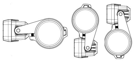
**4** Mount both brackets to the light using bolts, washers and key (avoid tightening firmly at this stage).
