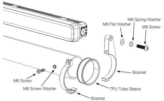
Note: The drawing only shows the mounting position above the bull bar
