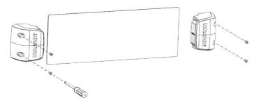
3 Insert 2 x Screw Cover into the screw hole of each lamp.
