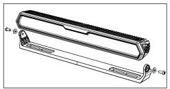
2 Remove M8 Torx screws and flat washers3 Remove lightbar from bracket
