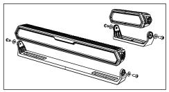
2 Remove M8 Torx screws and flat washers 3 Remove light bars from bracket
