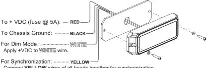
Connect **YELLOW** wires of all heads together for synchronization (All heads must be set at the same pattern)
